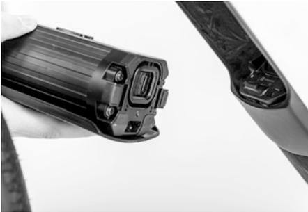
Finally, secure the drive battery in the down tube. To do this, put the key in the lock cylinder on the drive battery holder at the top end of the down tube on the left-hand side of the frame and turn it clockwise.
