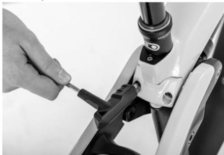
Figure 42: Wedge bolt/Dropper seat post
