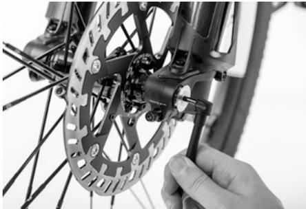
Figure 51: Fitting the clamping screws
