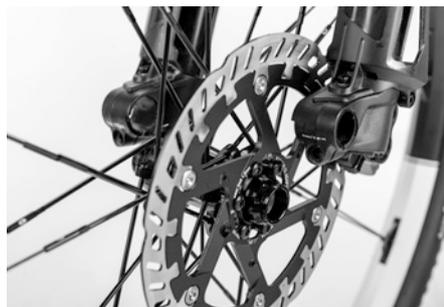
The front wheels of the PORSCHE eBike have bolted axles. When fitting the front hub, make sure that it is securely positioned in the dropout and that the brake disc is correctly centred in the brake calliper.
