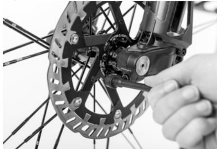
Figure 52: Inserting the breakdown tool
