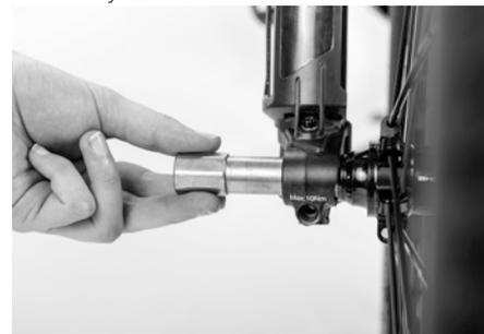
Tools are needed to remove the front wheel of the PORSCHE eBike Sport, in this case a Torx socket (size T25). Before you fit the axle, make sure that the thread is clean and undamaged. Push the lightly greased axle in from the right-hand side through the dropout and the hub until it reaches the stop.
