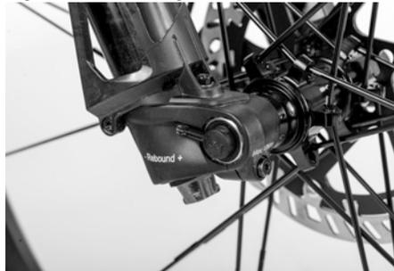
No tools are needed to remove the front wheel of the PORSCHE eBike Cross. Open the quick release lever on the axle and push the lightly greased axle through the hub until the thread engages with the dropout. Tighten the axle and apply the tension by turning the clamping lever upwards through 90°.
