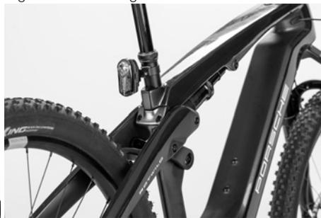
Both lights are supplied with suitable bolts. These must be tightened to a torque of 4 Nm.
