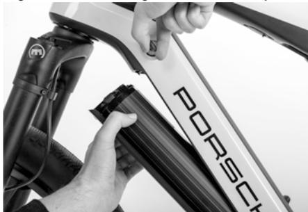
Figure 31: Removing the drive battery
