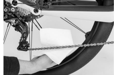
Figure 21: Lubricating the chain
