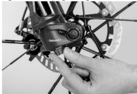
Too little damping will cause the fork to rebound very quickly. Too much damping will cause the suspension fork to bottom out during rapid consecutive impacts, because it can no longer rebound quickly enough.
