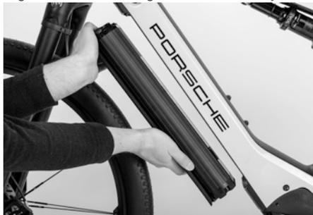
down tube as you will have to support this weight when the battery is released.
