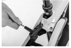
Figure 42: Wedge bolt/Dropper seat post
