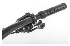
Figure 24: The position of the shifting lever (electronic)
