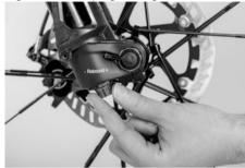
Too little damping will cause the fork to rebound very quickly. Too much damping will cause the suspension fork to bottom out during rapid consecutive impacts, because it can no longer rebound quickly enough.
