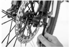
Figure 51: Fitting the clamping screws
