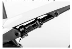
First of all, turn the red adjuster wheel anticlockwise until it reaches the stop. Then turn it clockwise in small stages/clicks until the shock damping is set correctly.
