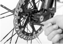
Figure 52: Inserting the breakdown tool
