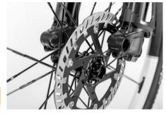
The front wheels of the PORSCHE eBike have bolted axles. When fitting the front hub, make sure that it is securely positioned in the dropout and that the brake disc is correctly centred in the brake calliper.
