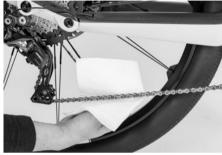
Figure 21: Lubricating the chain
