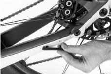
To fit the stand, position it on the inside of the chainstay in the slot intended for the purpose.
