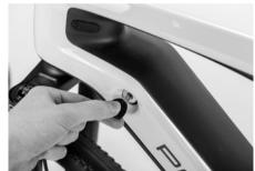
The drive battery is released from the lock mechanism in the down tube. A two-part locking plate holds the drive battery in position and prevents it from falling out. Press the two-part locking plate and remove the drive battery from the eBike.
