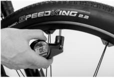
You should never let the tyre pressure exceed the maximum limit or fall below the minimum limit.
