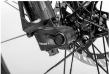
No tools are needed to remove the front wheel of the PORSCHE eBike Cross. Open the quick release lever on the axle and push the lightly greased axle through the hub until the thread engages with the dropout. Tighten the axle and apply the tension by turning the clamping lever upwards through 90°.
