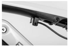
The charging process starts automatically. The charge status display flashes to indicate that the battery is being charged. The LED on the charger lights up to show that the charging process is under way.
