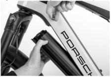
Figure 31: Removing the drive battery
