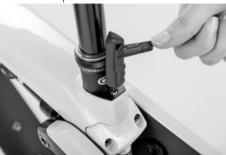
Check the tightening torques of the bolts on the through axle and the seat post (see "Recommended tightening torques").
