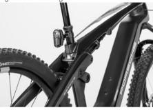
Both lights are supplied with suitable bolts. These must be tightened to a torque of 4 Nm.
