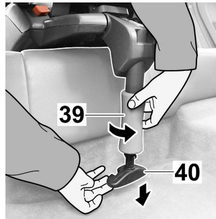
9. Turn the knob (39) counter-clockwise and pull the support leg (40) out until it rests securely on the vehicle floor. Then turn the knob in the opposite direction to lock.
