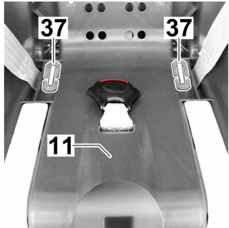
6. Pull out the Triglide (37) with which the belt is fastened at the bottom of the seat shell (11).
