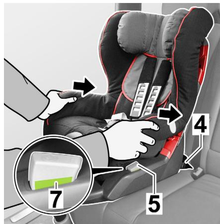
6. Push both locking arms (4) into the insertion aids until the locking arms engage on both sides with an audible “click”.
