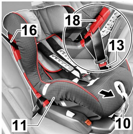
1. Push the adjusting handle (10) up and pull the seat shell (11) forward to the idle position.
