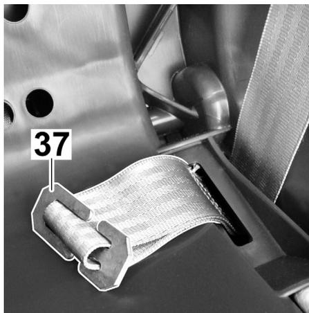
7. Push the belt loop back on the short side of the Triglode (37) and disengage the Triglode.
