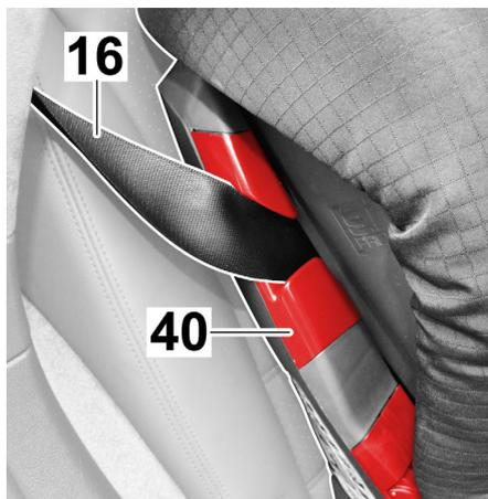
10. Place the diagonal belt (16) into the dark red belt guide (40) on the other side.
