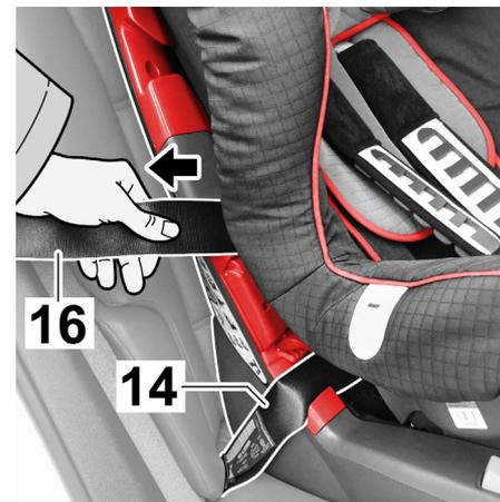
7. Tighten the lap belt (14) by pulling on the diagonal belt (16).
