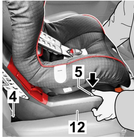
2. Press the grey locking buttons (5) on the left and right sides of the seat lower section (12). The locking arms (4) disengage.
