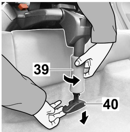
13. Turn the knob (39) counter-clockwise and pull the support leg (40) out until it rests securely on the vehicle floor. Then turn the knob in the opposite direction to lock.
