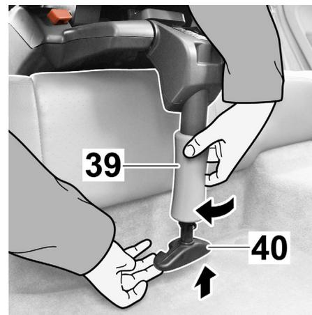
**Removing Child Seat with Three-Point Seat Belt**
