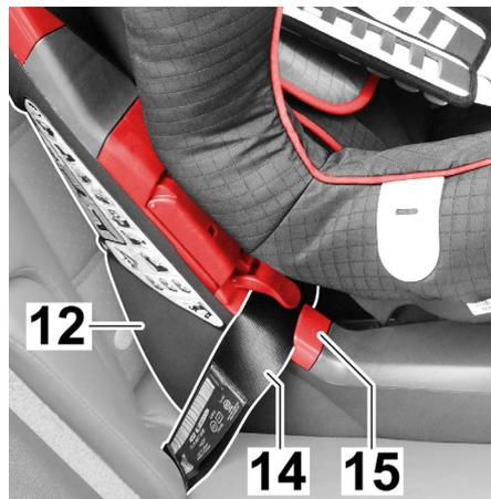
6. Place the lap belt (14) into the light red belt guides (15) on both sides of the seat lower section (12).
