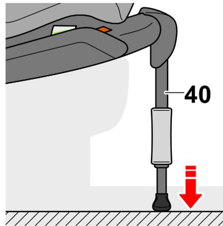
– the support leg rests securely on the vehicle floor without lifting the child seat off the vehicle seat surface.
