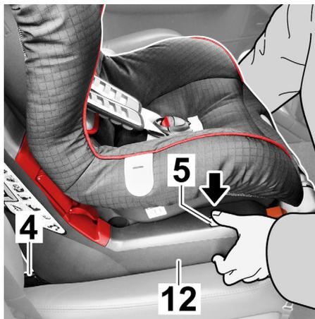
5. Press the grey locking buttons (5) on the left and right sides of the seat lower section (12).
