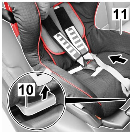
14. Push the adjusting handle (10) up and push the seat shell (11) back again.
