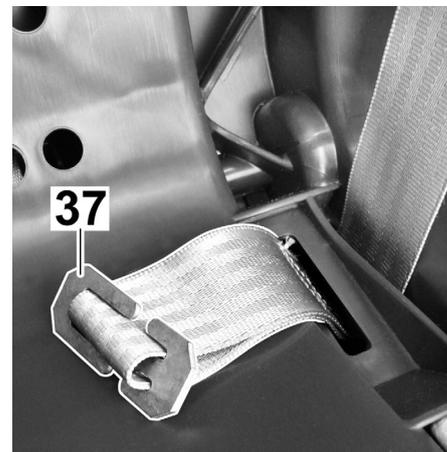
3. Engage the Triglode (37) in the long belt loop (engage the long side of the Triglode first, then the short side).
