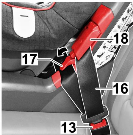
8. Swivel down the clamping lever (17) of the dark red belt clamp (18) on the side of the vehicle buckle (13).
