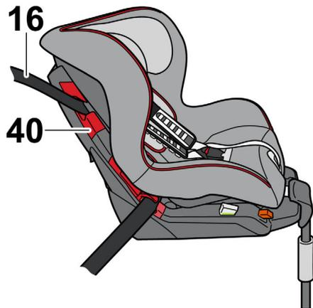
– the diagonal belt (16) passes through the dark red belt guide (40) located on the opposite side of the vehicle buckle.
