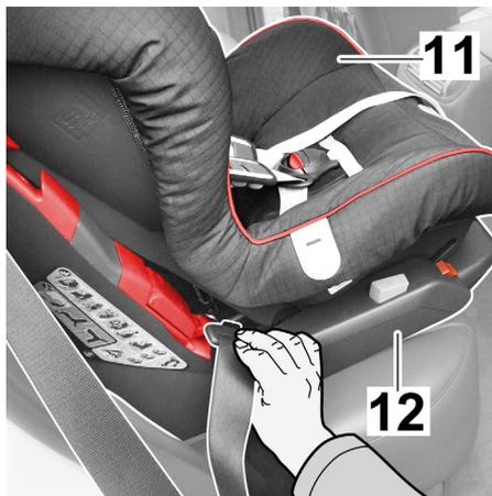
4. Pull the three-point seat belt out and guide it through between the seat shell (11) and the seat lower section (12).
