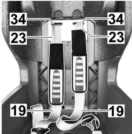
4. Pull the shoulder belts (19) and the belt loops of the shoulder pads (23) out of the belt slots (34).
