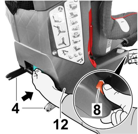
3. Press the orange tensioning button (8) and simultaneously push the locking arms (4) back into the seat lower section (12).
