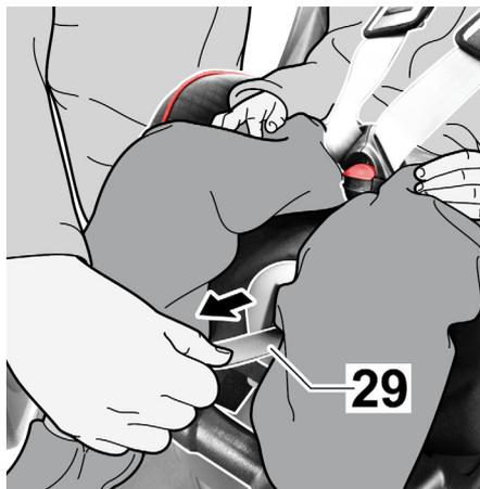
9. Tighten the belts until they are snug against the body. To do this, pull the belt end (29) out straight.
