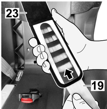
6. Thread the shoulder pads (23) onto the shoulder belts (19).
