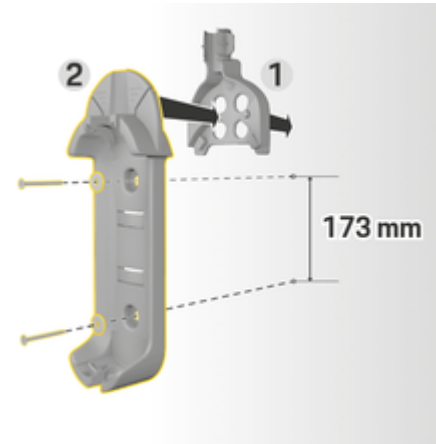
Fig. 3: Drilling dimensions
